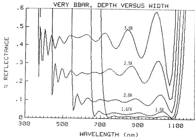
FIG. 1. VARIATION OF MINIMUM AVERAGE REFLECTANCE WITH BANDWIDTH FOR  $T = 3.0$  CYCLES.
