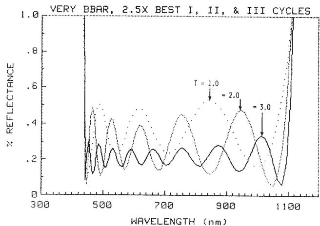
FIG. 2. VARIATION OF MINIMUM AVERAGE REFLECTANCE WITH OVERALL OPTICAL THICKNESS.
