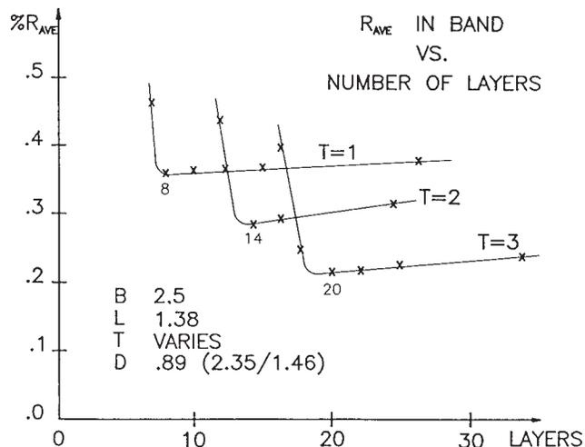
FIG. 5. AVERAGE REFLECTANCE IN BAND VERSUS NUMBER OF LAYERS. THIS IMPLIES  $\# = 2 + 6 \cdot T$  LAYERS. X'S ARE EMPIRICAL POINTS.
