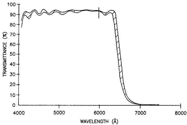
Fig. 2. Result of constant level monitoring error compensation from Zhao[3] when monitor wavelength (vertical bar) is near the edge of the passband.
