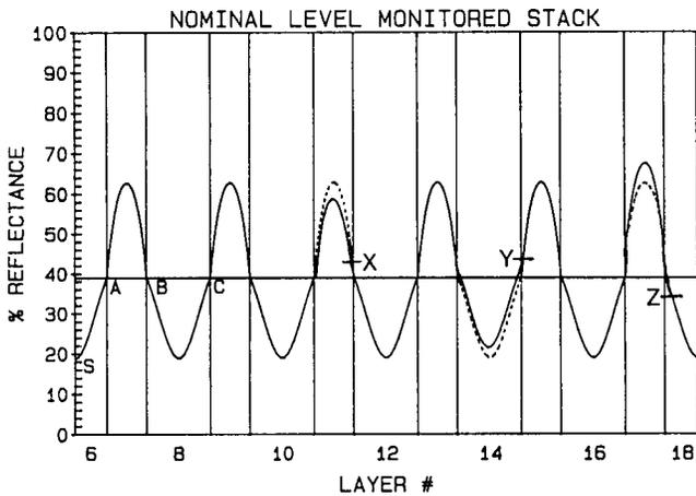
Fig. 5. Steering corrections (X, Y, & Z) for turning values that are too low (layer 11) or too high (layers 14 & 17).
