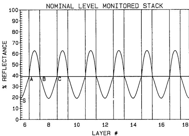
Fig. 4. Predicted optical monitor trace for constant level monitoring where each layer is terminated as its reflectance reaches the level as at points A, B, and C.
