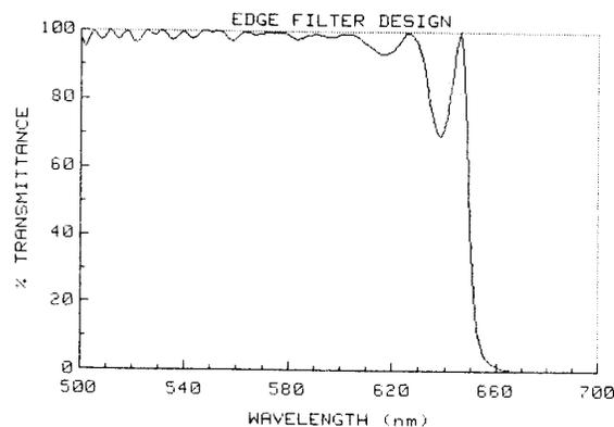
Fig. 1. Typical example of an edge filter design of the form discussed in this paper.
