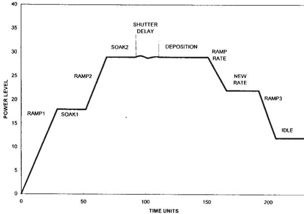
Fig. 4. Typical crystal controller power profile with time.
