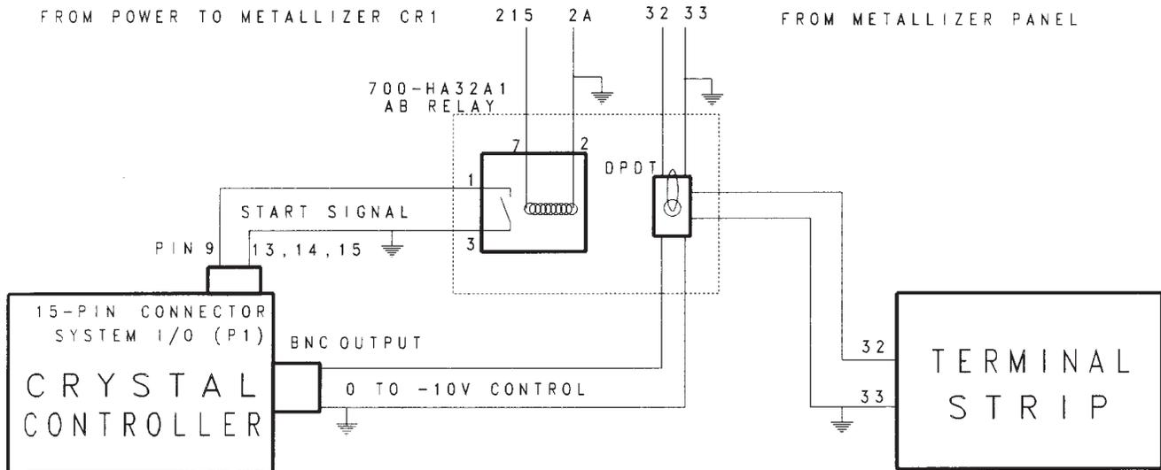
Fig. 5. Integration of the crystal controller to the metallizer. \* STC-200, Sycon Instruments, Inc., Syracuse, NY
