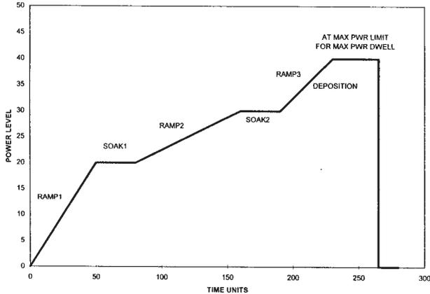
Fig. 6. Variables available to program in the controller.
