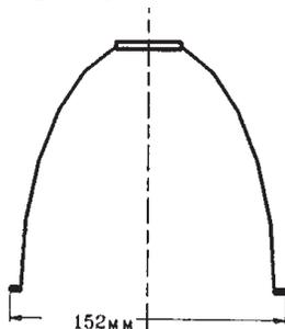
Fig.1. Cross section of a deep cavity reflector part.
