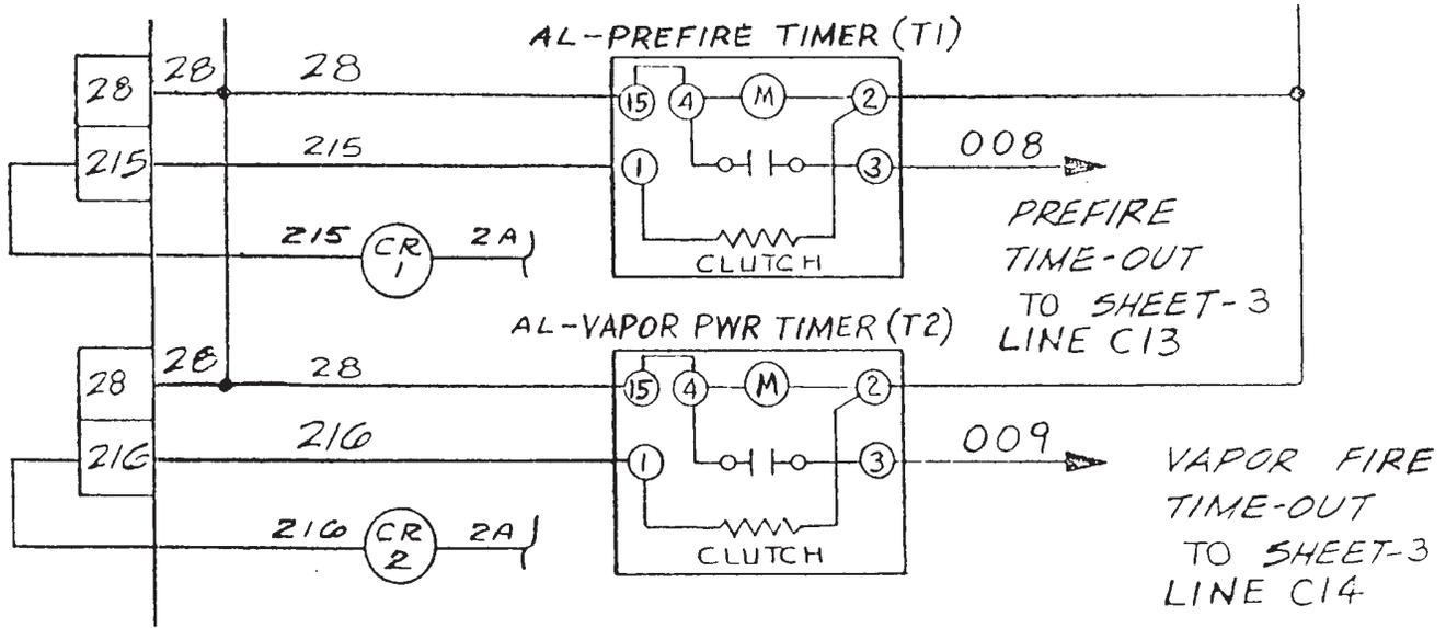
Fig. 2. Timing control section of metallizer ladder logic.
