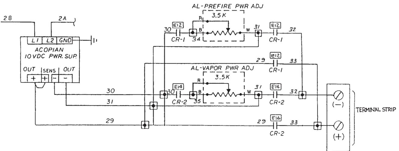
Fig. 3. Voltage control section of metallizer ladder logic.
