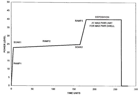
Fig. 7. Program simulating original timers and powers.
