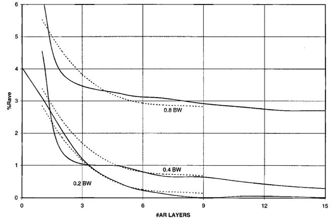
Figure 10. Solid lines are %Rave for LWP filters from the individual detail designs versus layers and bandwidth. The dotted lines are the values predicted by the equations.
