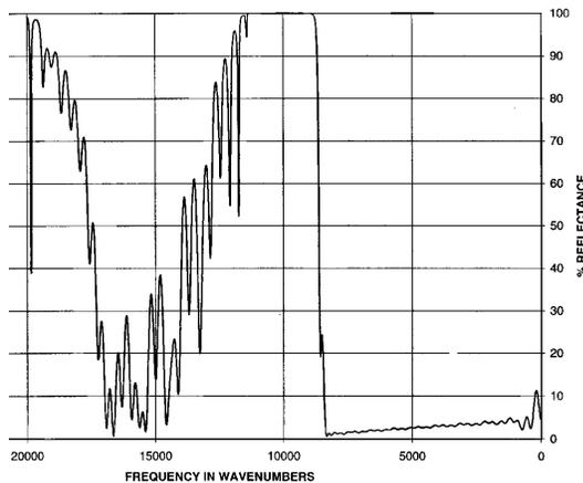
Figure 4. Results of a LWP design where the bandwidth was 0.8 and the total number of additional layers was 19.
