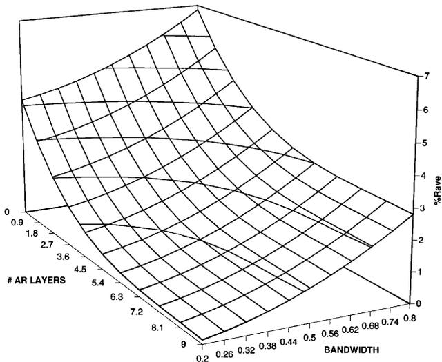
Figure 9. Three dimensional plot of the resulting minimum predicted %Rave versus number of AR layers and bandwidth for the LWP filters.
