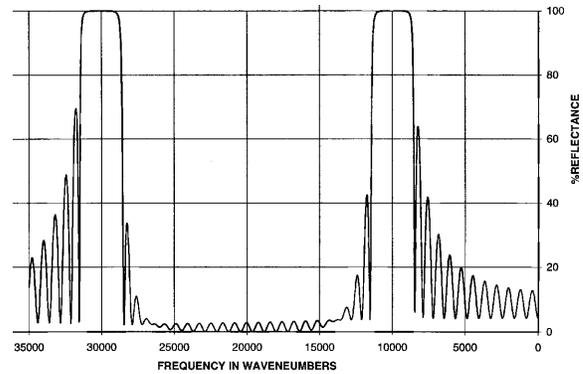
Figure 5. SWP design for the 1.6 maximum bandwidth using 11 additional AR layers.
