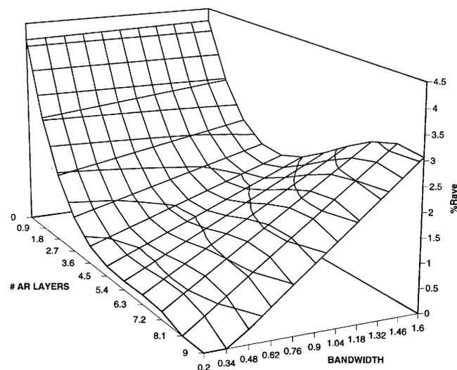
Figure 7. Three dimensional plot of the resulting minimum predicted %Rave versus number of AR layers and bandwidth for the SWP filters.
