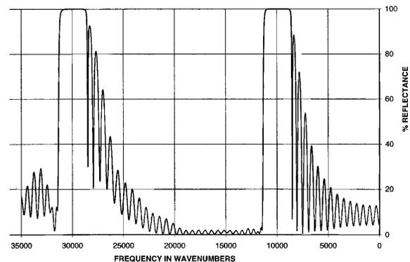
Figure 6. SWP designed for half (0.8) of the maximum bandwidth using 11 additional AR layers.
