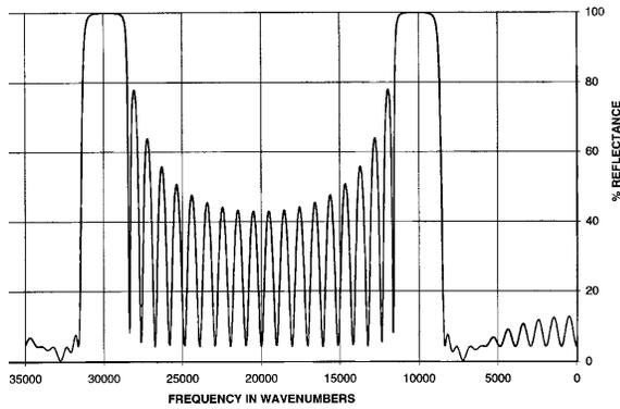
Figure 3. Long wavelength pass (LWP) filter on a linear frequency scale.
