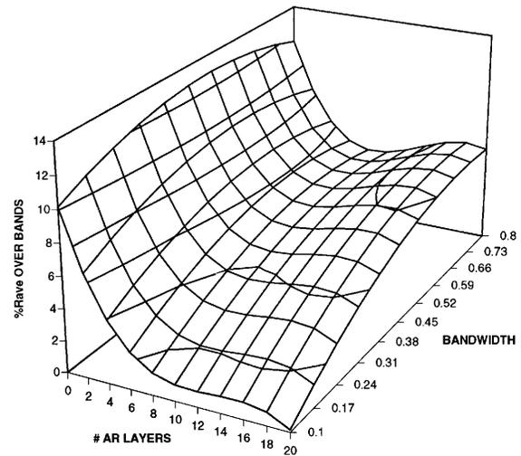
Figure 11. Three dimensional plot of the resulting minimum predicted %Rave versus number of AR layers and bandwidth for the BWP filters.
