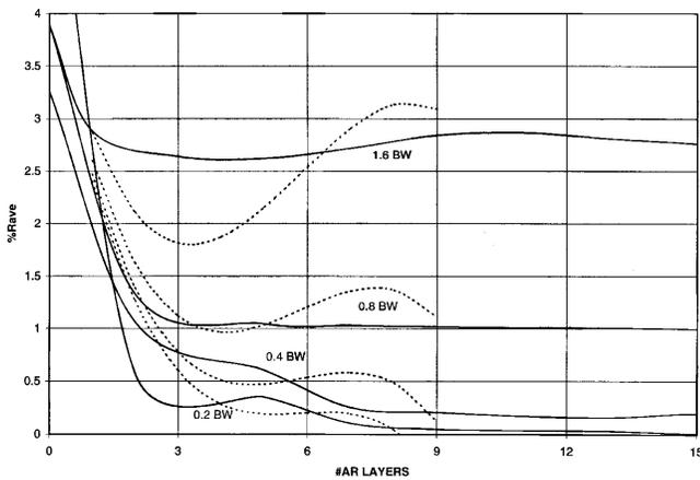
Figure 8. Solid lines are %Rave for SWP filters from the individual detail designs versus layers and bandwidth. The dotted lines are the values predicted by the equations.
