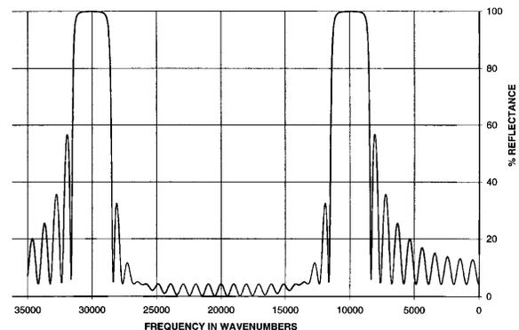
Figure 2. Short wavelength pass (SWP) filter on a linear frequency or wavenumber ( $\text{cm}^{-1}$ ) scale.
