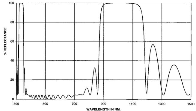
Figure 1. Short wavelength pass (SWP) filter on a linear wavelength scale.
