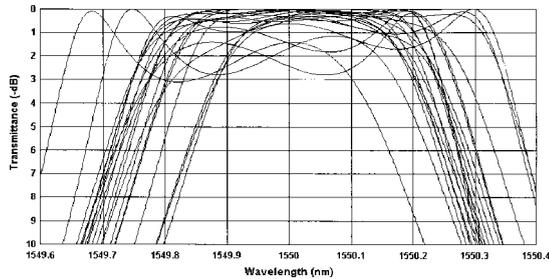
Fig. 1. Uncompensated random errors of 0.01% in the optical thickness of layers in the 114-layer, three-cavity filter given in the text. Note that transmittance scale is  $10\times$  that of Figs. 2–7.
