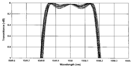
Fig. 3. Effects of 1% simulated random errors centered about the turning points when terminating the layers (monitoring) in a mode that provides compensation.
