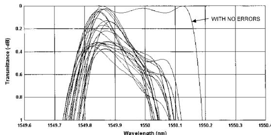
Fig. 7. Effects of 3% random compensated errors that occur entirely before the turning point, for comparison with the results in Figs. 6.
