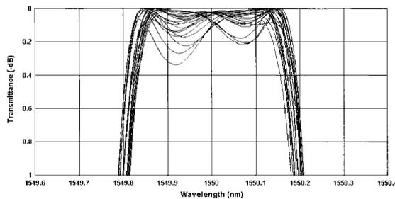
Fig. 2. Uncompensated random errors of 0.002% in a filter as shown in Fig. 1.
