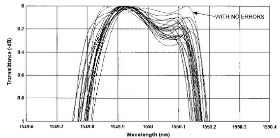
Fig. 6. Effects of 3% random compensated errors that extend only from the turning point to the greater thickness, for comparison with the results in Figs. 4 and 5.
