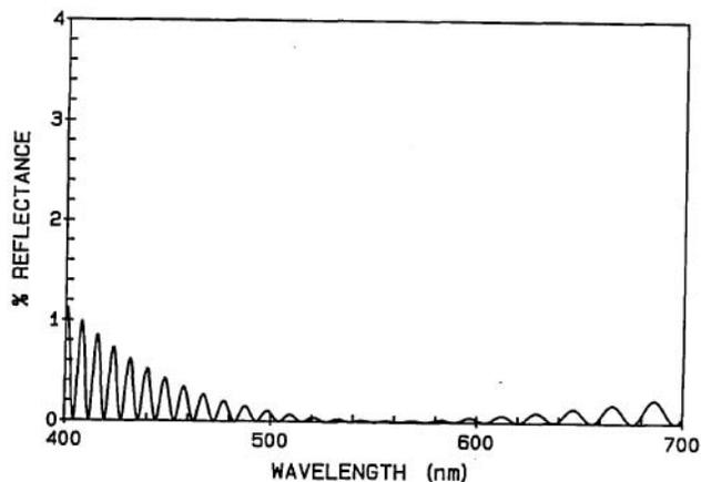
Fig. 3. Interface reflection of surfaces as in Fig. 1, which have been coated with a QWOT of 1.64 index at 550 nm prior to cementing.
