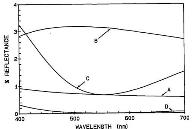
Fig. 2. Curve A, Fresnel reflection at the interface between 1.785 glass (SF11) and 1.52 cement. Curve B, reflection of the surface as in curve A if coated with one QWOT of magnesium fluoride. Curve C, reflection of the surface as in curve A if coated with two QWOTs of magnesium fluoride. Curve D, reflection of surface as in curve A if coated with one QWOT of aluminum oxide (1.64 index).
