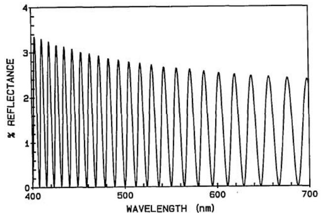
Fig. 1. Interface reflection of surfaces of high index (1.785) glasses SF11 and LaK21, which have been cemented with thirty waves of optical thickness 1.52 index cement.
