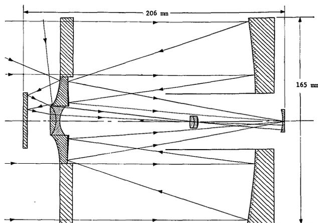
Fig. 4. Combined optical system.
