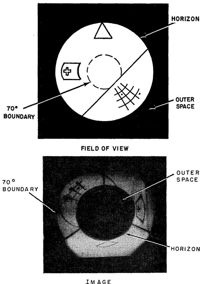
Fig. 3. Space sextant monitor display of field of view as seen by image tube through the wide-field system.
