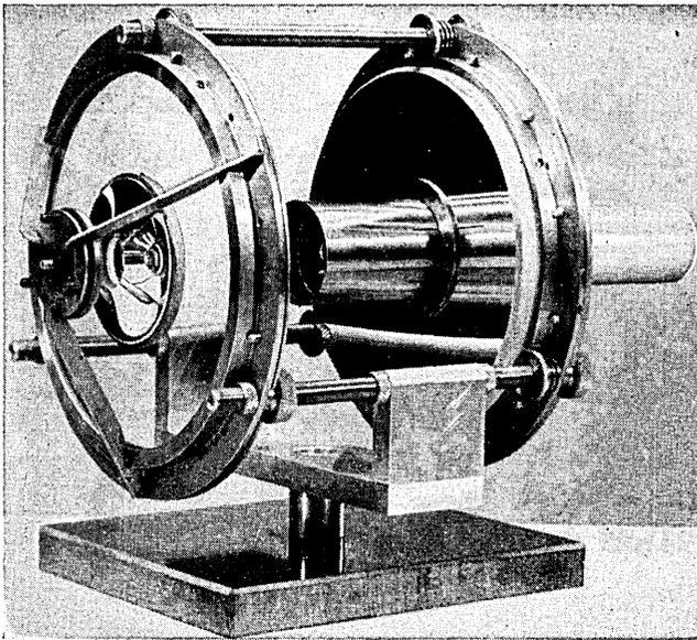
Fig. 5. Dual-field star tracker with image tube shield.
