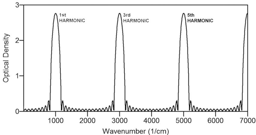
Fig. 2. A QWOT stack design with its fundamental blocking band at  $1000\text{ cm}^{-1}$  and harmonics at 3, 5, 7, etc., of that frequency. There are no bands less than  $1000\text{ cm}^{-1}$  (LWP side).
