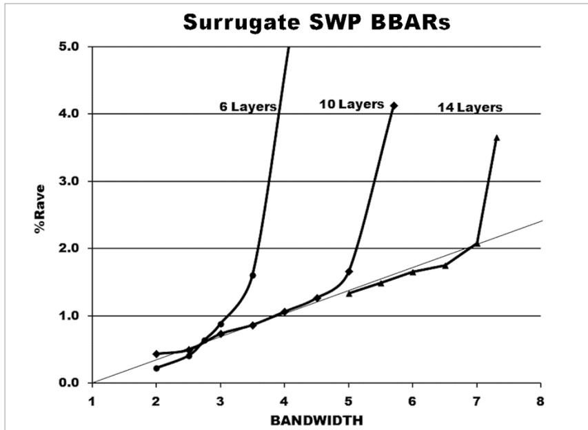
Fig. 12. Average reflectance in a passband versus bandwidth for designs of 6, 10, and 14 layers per cycle which suppress the 3<sup>rd</sup>, 5<sup>th</sup>, and 7<sup>th</sup> harmonics respectively.
