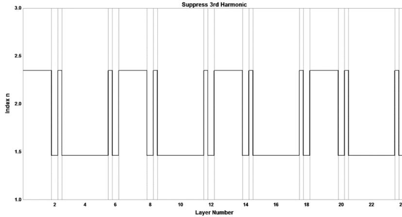
Fig. 6. Index versus thickness profile of symmetric layer stack with 6 layers per cycle. This gives blocking bands at harmonics 1, 5, 7, etc., but **NOT** at the 3<sup>rd</sup> harmonic, as seen in Fig. 7.
