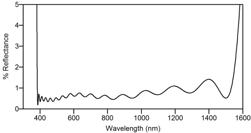
Fig. 1. A broadband AR coating started from a QWOT stack at about 310 nm. This could be extended to the right as much as needed with a tradeoff in the average reflectance percentage (Rave) in the band.
