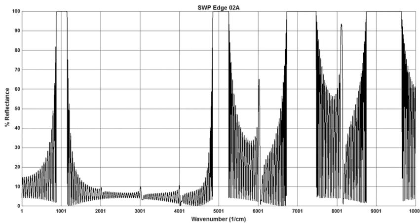
Fig. 7. Blocking- and pass-bands produced by the index versus thickness profile of Fig. 6.
