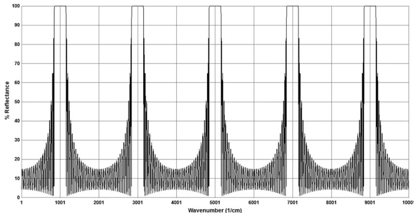
Fig. 5. Blocking- and pass-bands produced by the index versus thickness profile of Fig. 4.
