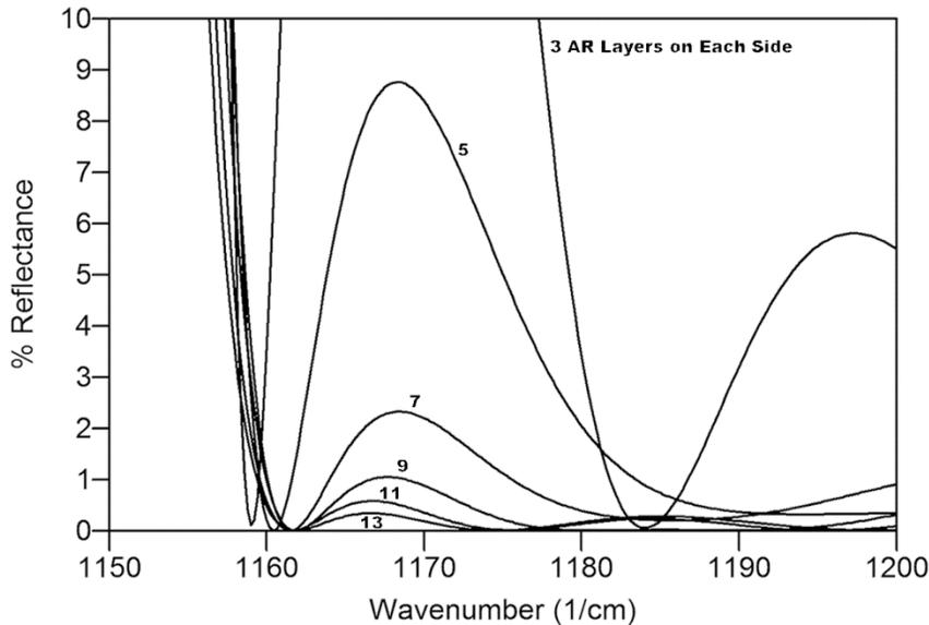
Fig. 15. Squareness between the band edge and passband as a function of the number of AR layers on each side of the blocking band stack.
