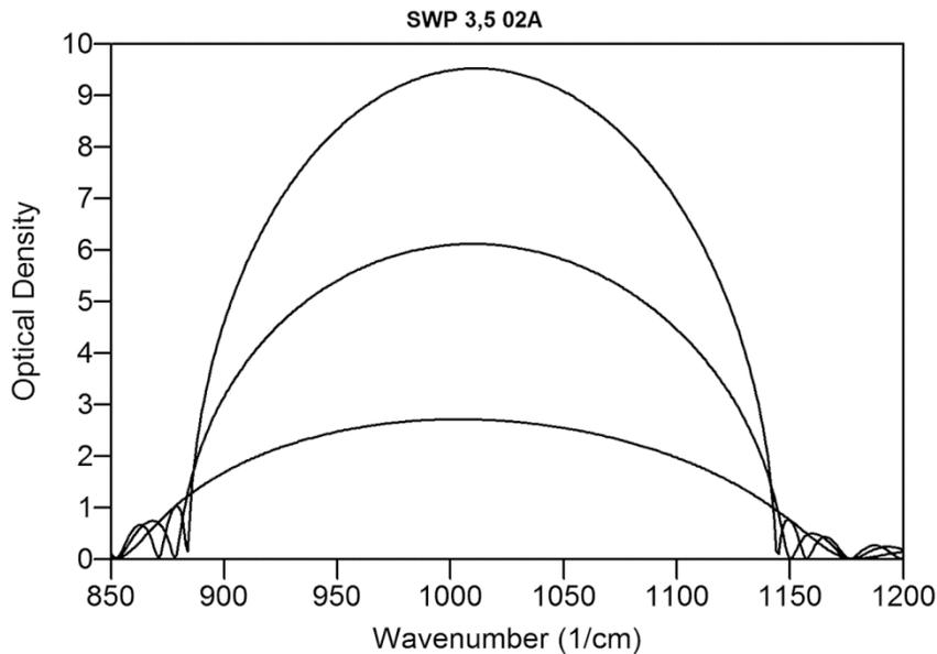
Fig. 14. Blocking optical density of the 1<sup>st</sup> harmonic for the designs of Figs. 10-11 (suppressed 3<sup>rd</sup>, 5<sup>th</sup>, and 7<sup>th</sup> harmonics) with 10, 20, and 30 layer cycles in the designs. The height is greatest for the design of 30 cycles and progressively lower 20 and 10 layer cycles.
