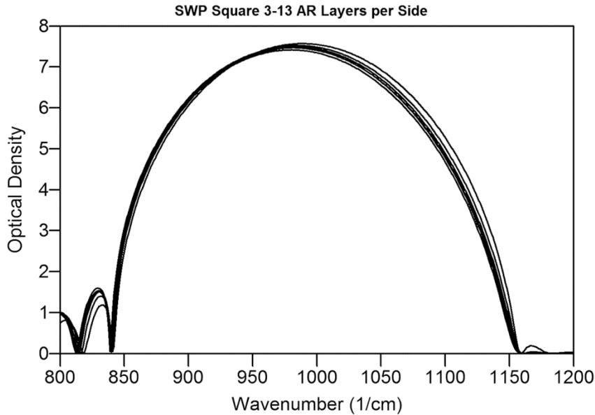
Fig. 16. Steepness of the band edge and passband as a function of the number of AR layers on each side of the blocking band stack.
