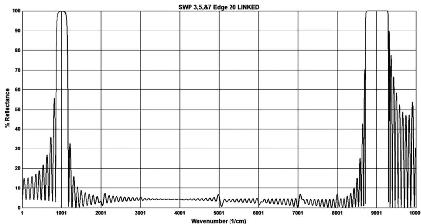
Fig. 11. Blocking- and pass-bands produced by the index versus thickness profile of Fig. 10.
