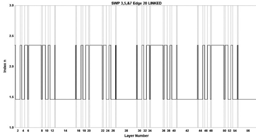
Fig. 10. Index versus thickness profile of symmetric layer stack with 14 layers per cycle. This gives blocking bands at harmonics 1, 9, etc., but **NOT** at the 3<sup>rd</sup>, 5<sup>th</sup>, and 7<sup>th</sup> harmonics, as seen in Fig. 11.
