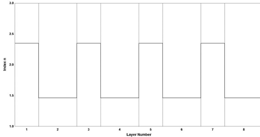
Fig. 4. Index versus thickness profile of QWOT stack with 2 layers per cycle. This gives blocking bands at all odd harmonics (1, 3, 5, 7, etc.), but NOT at the even harmonics, as seen in Figs. 2 and 5.
