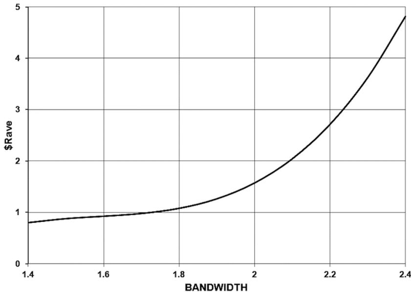
Fig. 3. Estimated potential Rave versus Bandwidth in a QWOT stack SWP edge filter.
