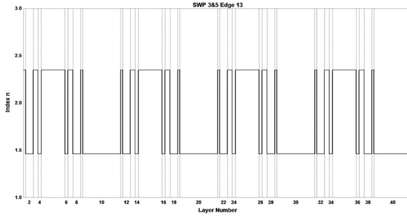
Fig. 8. Index versus thickness profile of symmetric layer stack with 10 layers per cycle. This gives blocking bands at harmonics 1, 7, etc., but **NOT** at the 3<sup>rd</sup> and 5<sup>th</sup> harmonics, as seen in Fig. 9.
