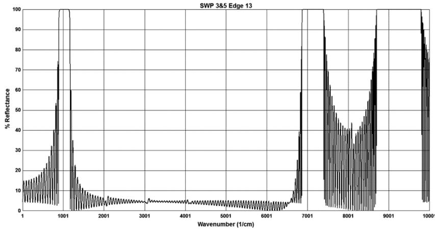
Fig. 9. Blocking- and pass-bands produced by the index versus thickness profile of Fig. 8.
