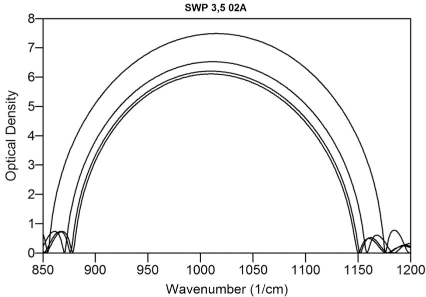
Fig. 13. Blocking optical density of the 1<sup>st</sup> harmonic band for the designs of Figs. 4-5, 6-7, 8-9, and 10-11. The width is greatest for the QWOT design of 2 layers per cycle and progressively narrower with increasing numbers of layers per cycle.
