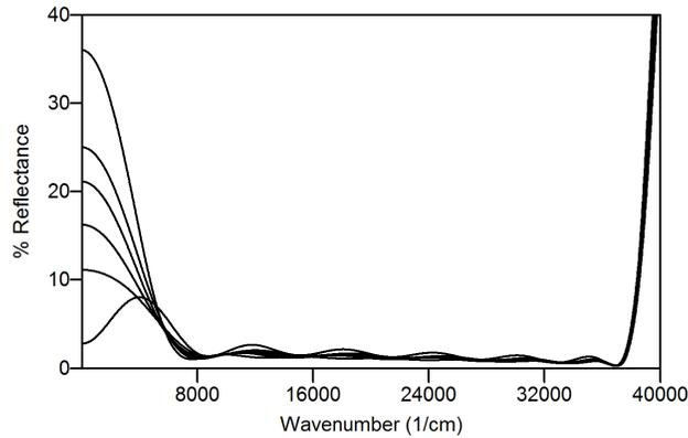
Figure 5. Reflectance versus wavenumber in the AR band  $6250\text{-}37500\text{ cm}^{-1}$  for the step-down of Fig. 4 and for substrates of lesser indices, down to below a threshold which results in a non-step-down design.
