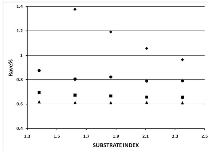
Figure 11. Average reflectance in the AR band of  $B = 4$  versus substrate index of refraction for  $\frac{1}{2}$  cycle (step-down) designs (diamonds), one cycle designs (round dots), two cycle designs (squares), and three cycle designs (triangles).
