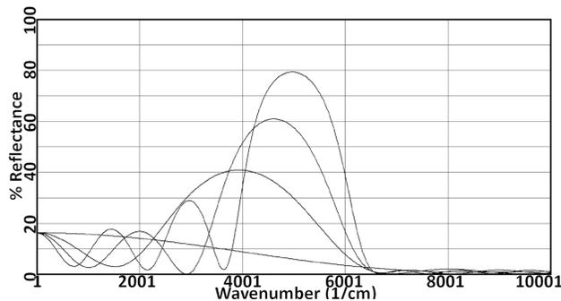
Figure 6. Reflectance versus wavenumber of optimized designs on a high index of refraction substrate (2.35), showing a step-down ( $\frac{1}{2}$  cycle), 1- $\frac{1}{2}$  cycle, 2- $\frac{1}{2}$  cycle, and 3- $\frac{1}{2}$  cycle design.
