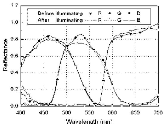
Figure 4. Typical blue, green, and red pixel filters<sup>8</sup>.
