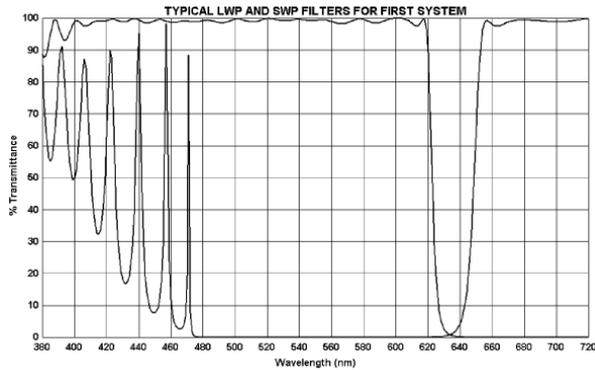
**Figure 6.** Short wave pass filter for display at ~620 nm and long wave pass at ~650 nm for NVIS used in First Approach.
