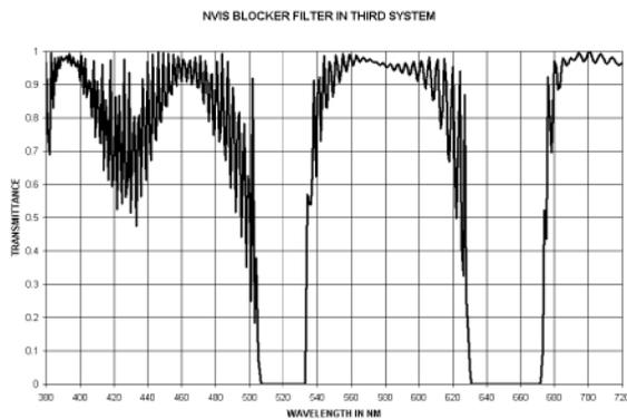
**Figure 12.** Multilayer filter for NVIS in Third Approach.
