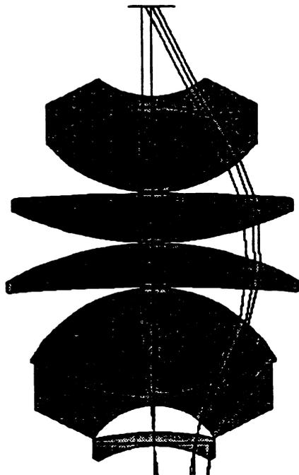
Fig. 1. A good eyepiece design until the effect of cement between the doublets was taken into account. Then TIR occurred at the cemented interfaces.
