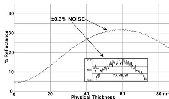
Fig. 4. A typical raw optical monitor signal with  $\pm 0.3\%$  noise. The inset is a 7X expansion of the region around the TP with  $0.3\%$  vertical chart intervals to illustrate the scope of the noise.
