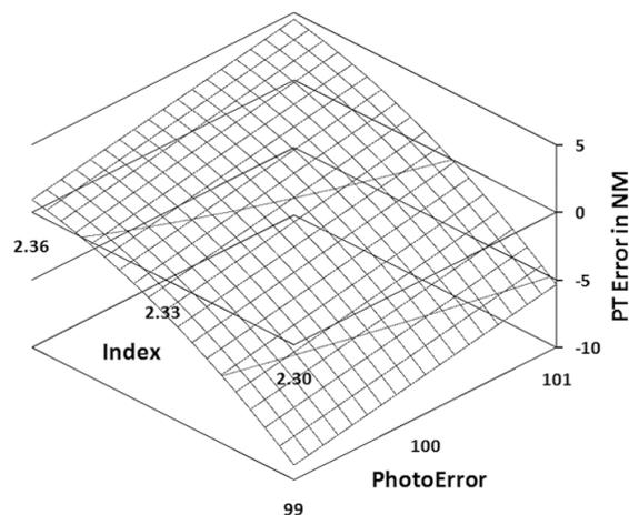
Fig. 2. Physical thickness error as a function of index of refraction variations and photometric scale error when using the LEVEL CUT strategy.
