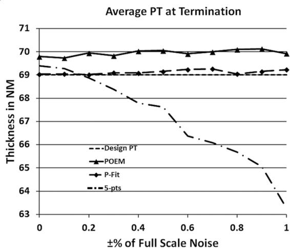
Fig. 10. Results of the average thickness error versus noise at the termination for the three strategies with 5% POE and a TP at  $\sim 31\%R$ . The design thickness of 69 nm is plotted as a dotted line.
