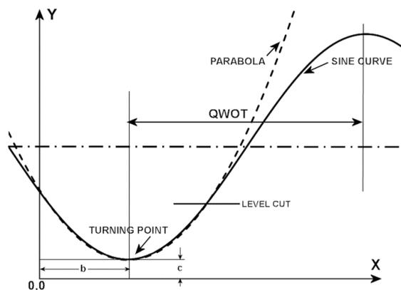
Fig. 3. A parabolic curve matches the sine curve in the region of a TP. The  $b$  and  $c$  constants define the position of the vertex of the parabola (TP) with respect to the origin. A Level Cut is also illustrated at a specified photometric level .
