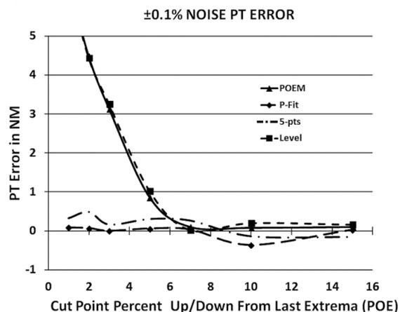
Fig. 6. Systematic physical thickness errors in nm versus cut point position (POE) with  $\pm 0.1\%$  noise using the four different termination strategies.
