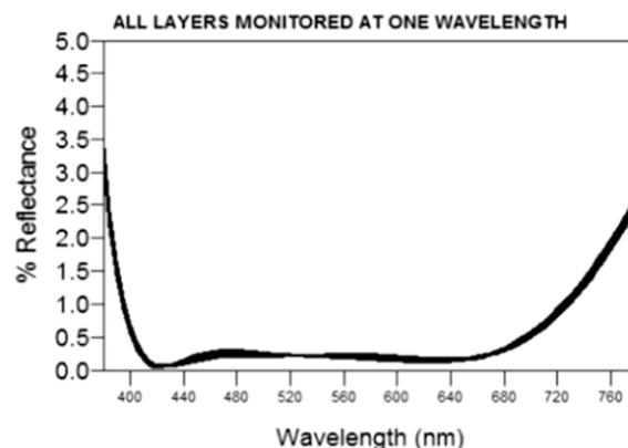
Fig. 16. Results of ten runs each with random noise at the wavelengths from 380 nm with the strategy for each layer of 4333 and the noise percentage of  $\pm 0.1$ . The other strategies and wavelengths shown in Fig. 15 look essentially the same at this noise level
