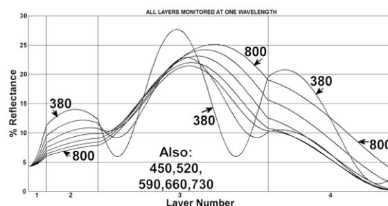
Fig. 14. Simulated optical monitor signal for this 4-layer BBAR at each of the wavelengths studied from 380 to 800 nm.
