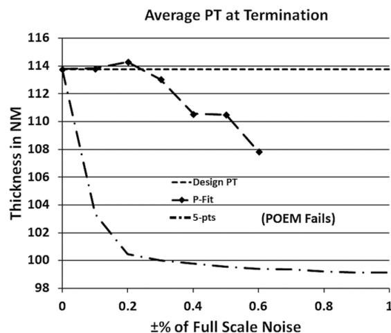
Fig. 12. Results of the average thickness error versus noise at the termination for the two TP strategies with 5% POE and a TP at 1.26%R. The POEM fails in this case. The design thickness of 113.74 nm is plotted as a dotted line.
