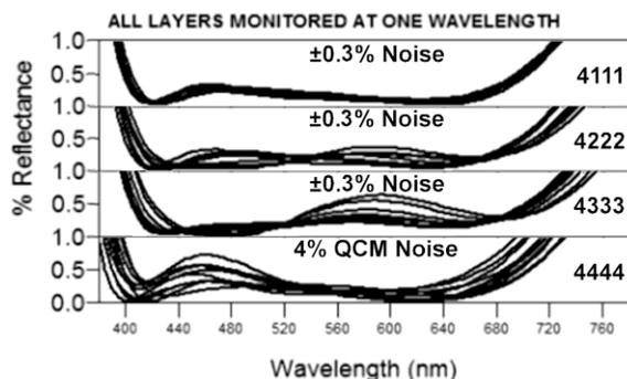
Fig. 17. Performance at 380 nm of the four termination strategies with  $\pm 0.3\%$  full scale noise for POEM (4111), TP via P-Fit (4222), TP using 5-pts (4333), and QCM (4444) with 4% random errors.
