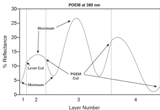
Fig. 1. A computer simulated monitoring curve of %R versus physical thickness monitoring at 380 nm in reflectance for the 4-layer AR.
