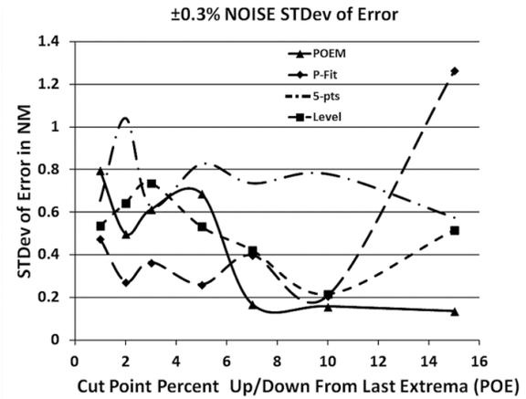
Fig. 9. Standard deviation of the PT error in nm from the data runs in Fig. 8 versus cut point position with  $\pm 0.3\%$  noise.
