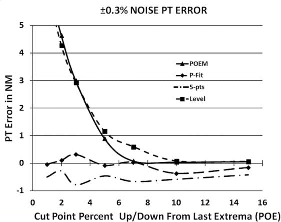
Fig. 8. Systematic physical thickness error in nm versus cut point position with  $\pm 0.3\%$  noise.
