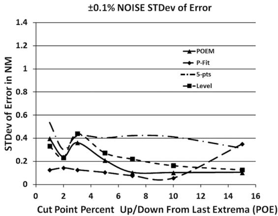
Fig. 7. Standard deviation of the PT error in nm from the data runs in Fig. 6 versus cut point position with  $\pm 0.1\%$  noise.
