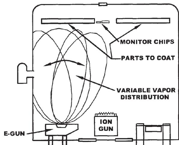
Figure 1: The variable distribution of silicon dioxide evaporant from an E-gun as is commonly experienced in physical vapor deposition.
