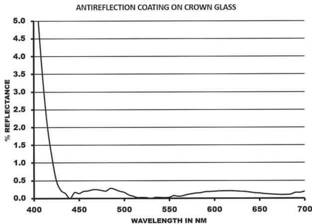
Figure 4: Spectral reflectance of AR coating using process described.
