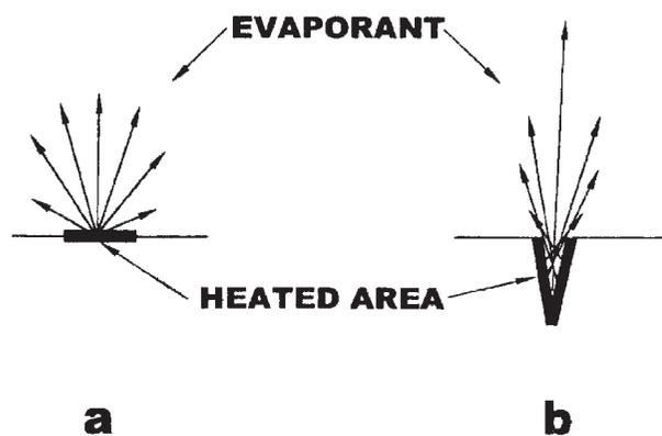
Figure 2: The vapor distribution of silicon dioxide evaporant from a flat surface of  $\text{SiO}_2$  versus a groove or tunnel where the radiant heat is confined and causes extra heat and a higher evaporation rate.
