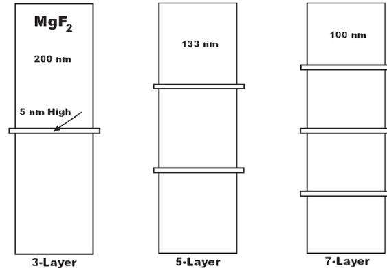
Figure 5: Layer structures of 400 nm stacks of  $\text{MgF}_2$  with 5 nm layers of Dralo inserted.
