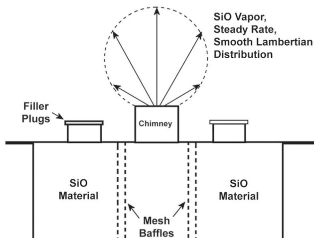
Figure 3: The vapor distribution of silicon monoxide from a resistance source is Lambertian, steady, and reproducible.
