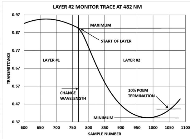
Figure 6. Optical monitor trace at 482 nm of layer #2 in the filter design of Figs. 1 and 2.
