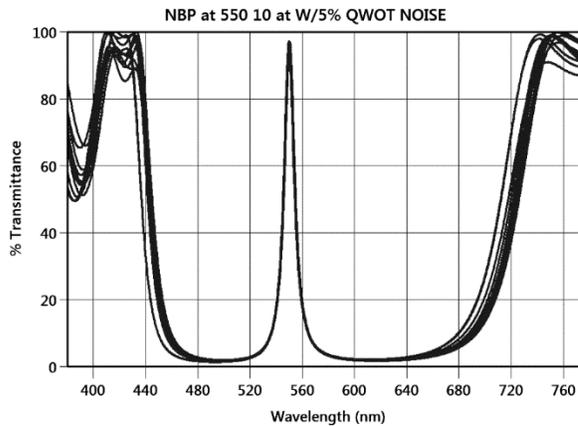
Figure 4. Spectral plot of 10 cases of the filter in Figure 1 and 2 with random  $\pm 5\%$  QWOT errors in each layer, but where “turning point” monitoring was used giving error compensation.
