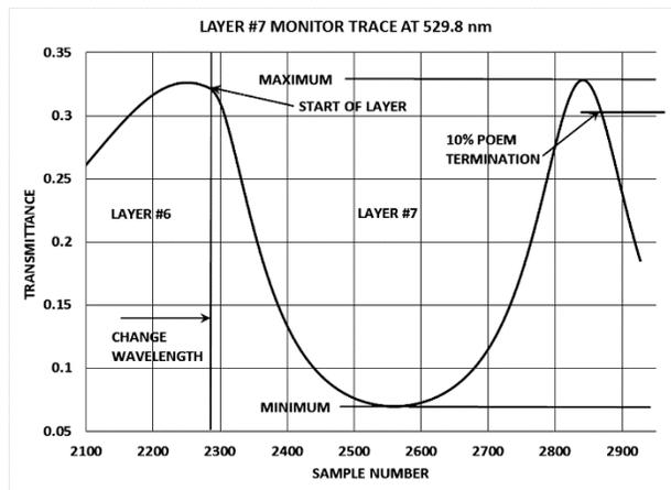
Figure 5. Optical monitor trace at 529.8 nm of layer #7 in the filter design of Figs. 1 and 2.
