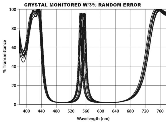
Figure 3. Spectral plot of 10 cases of the filter in Figure 1 and 2 with random  $\pm 3\%$  uncompensated errors in each layer.
