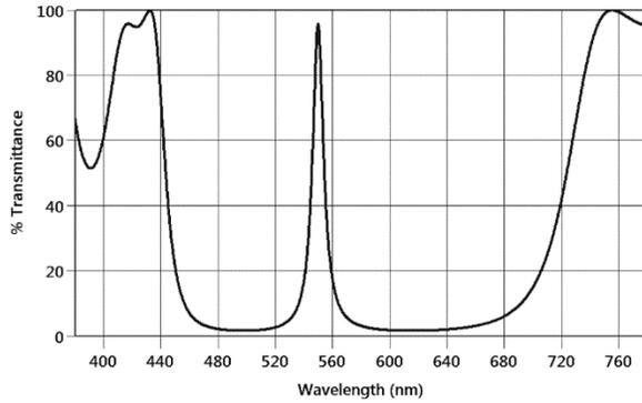
Figure 2. Spectral plot of the 13-layer NBP filter of Figure 1.
