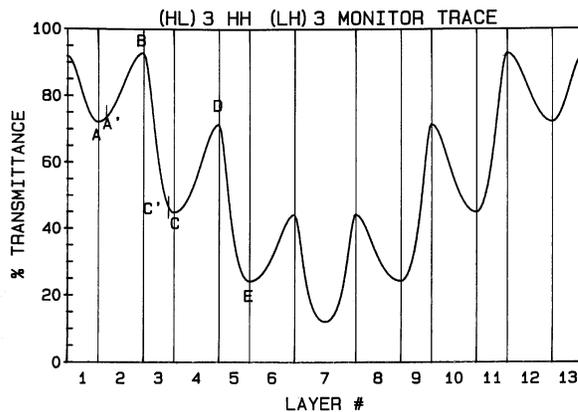
Figure 1. Optical monitor trace of a 13-layer NBP filter at 550 nm as in Figure 2. The ideal layer terminations are at A, B, C, D, E, etc., while errors are shown at A' and C' which are partially compensated by terminating the next layer at the next turning point.
