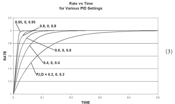
Figure 3. Various PID settings with critical damping showing relative response times.
