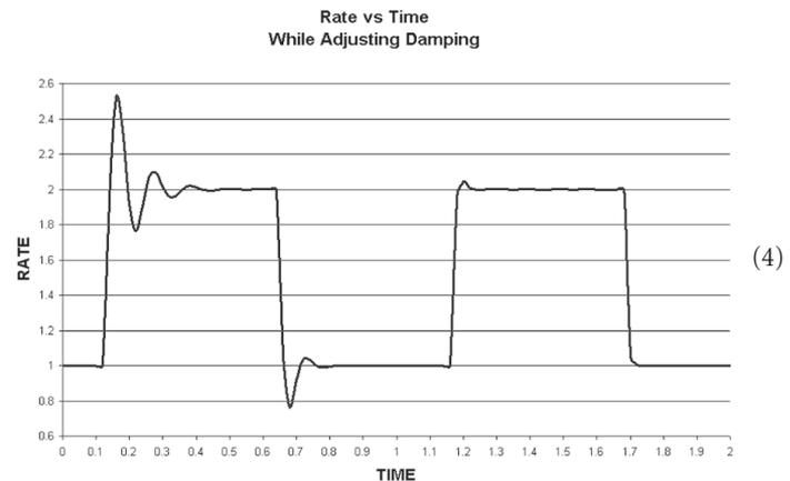
Figure 4. Adjusting damping to higher values to reduce overshoot and "ringing."
