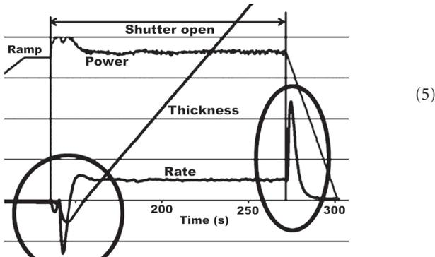
Figure 5. Real data with the transient effect for a standard "AT" cut quartz crystal..
