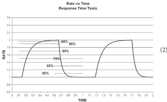
Figure 2. Testing the non-controlled response time for changes between 50% and full rate.
