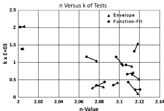
**Fig. 6.** Comparison of envelope and function fitting methods for finding  $n$  and  $k$  from %T spectra of optical coatings.
