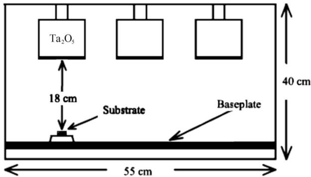
Fig. 1. Equipment configuration for the RF sputtering of  $\text{Ta}_2\text{O}_5$ .
