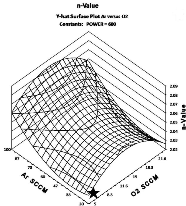
Fig. 3. Real part of index of refraction,  $n$ , derived from the reduction of the DOE data.
