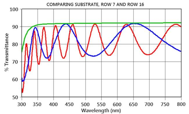
Fig. 4. Comparison of transmittance of the uncoated substrate, the thin, low-rate lowest  $k$ -value sample (#7), and the chosen higher-rate process (#16).
