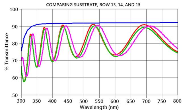
Fig. 5. Comparison of transmittance of the uncoated substrate and the three repeated runs to show run-to-run variations.
