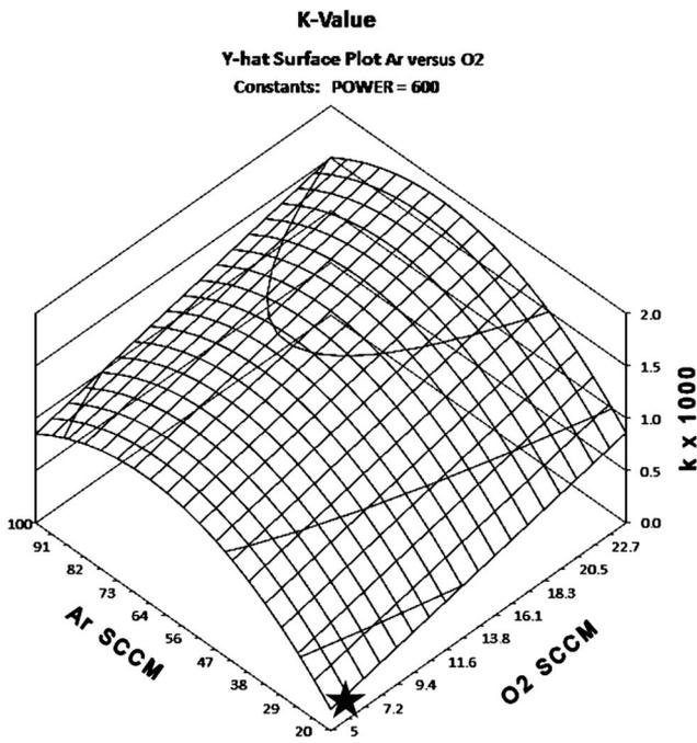
Fig. 2. Absorptance,  $k \times 1000$ , derived from DOE data reduction.
