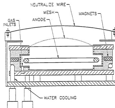
Figure 1 Cold Cathode Source tested.
