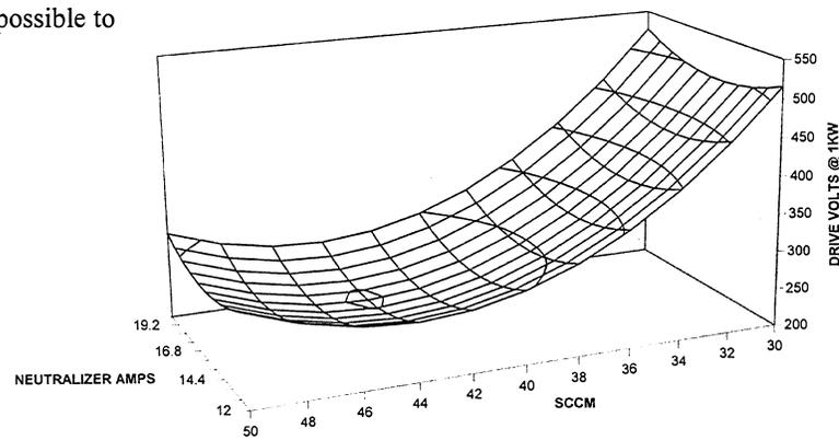
**Figure 7** Drive volts as a function of gas flow in SCCM and  $A_N$  for a 25% argon in oxygen gas mix.
