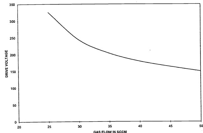
**Figure 3** Drive volts versus gas flow at 10 amps drive current, A<sub>D</sub>. In order to have not sparking, A<sub>N</sub> had to be 15.5 at 25 SCCM and 16.1 at 50 SCCM.
