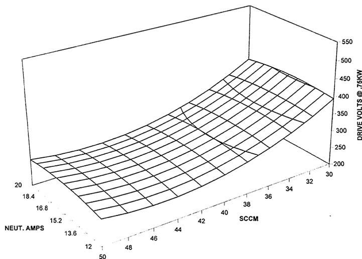
Figure 9 Drive volts as a function of gas flow in SCCM and A<sub>N</sub> with 50% argon and 50% oxygen by weight at .75 kilowatts of drive power.
