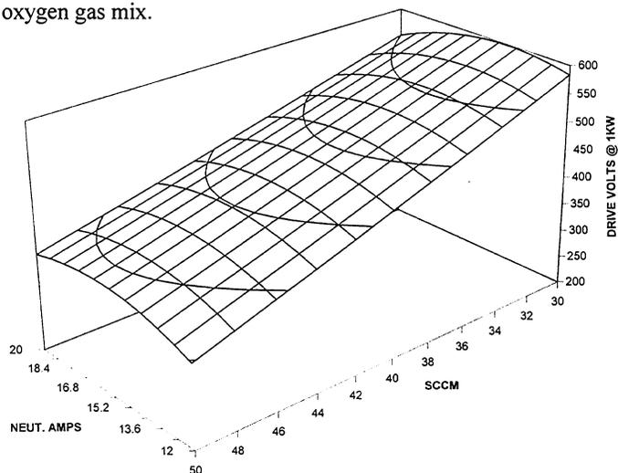
**Figure 8** Drive volts as a function of gas flow in SCCM and  $A_N$  with pure oxygen (0% argon) at 1 kilowatt of drive power.
