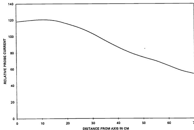
Figure 4 Ion probe readings versus position off-axis in a flat plane perpendicular to the source axis at 60 cm from the source for 26 SCCM, 10  $A_D$ , 310  $V_D$ , and 16.0  $A_N$ .
