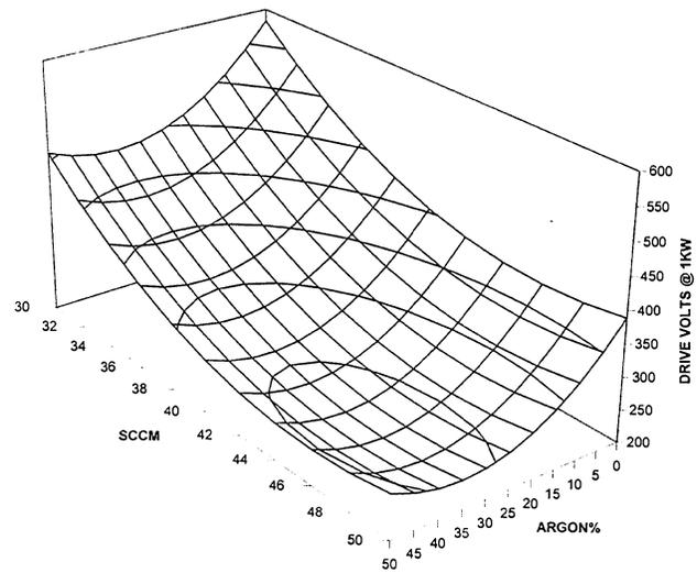
**Figure 6** Drive volts as a function of % argon mixed with oxygen and gas flow in SCCM at 1 kilowatt input power.
