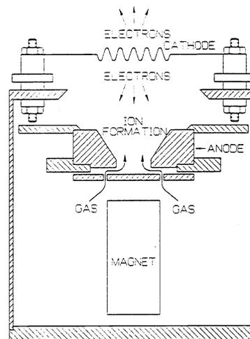
Figure 2 End-Hall Source tested.
