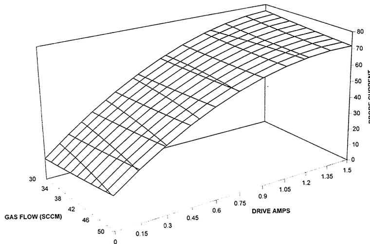
Figure 5 Probe current versus drive current and gas flow of IS1000.
